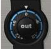
The Output knob allows you to increase or decrease the output level to compensate for any level changes caused by PSP Neon’s filtering. Clicking and dragging the knob to the right or upward increases the gain. Clicking and dragging the knob to the left or downward decreases the gain.
