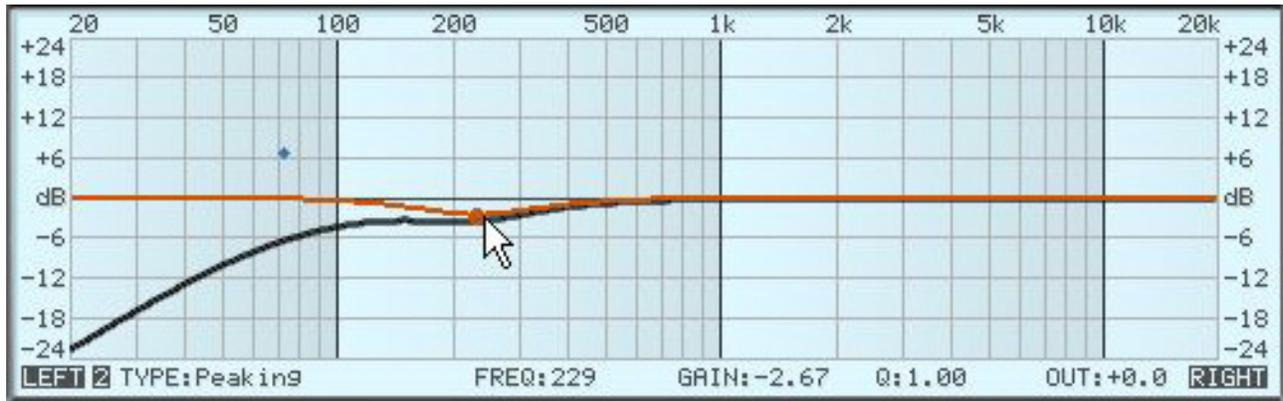
The upper third of PSP Neon's interface consists of the EQ graph. It offers you a graphic representation of the plug-in's filtration curve, with the x-axis displaying frequency in Hz, and the y-axis displaying gain in dB.
