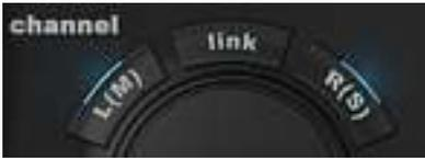
When using a stereo or mid-side instance of PSP Neon HR, you choose to process each channel independently or as a linked pair. These three buttons determine which channel is being edited.
